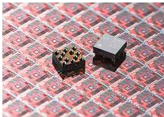
Figure 6. Bosch BMC 150 three axis magnetic sensor in a 2x2mm WLP.
