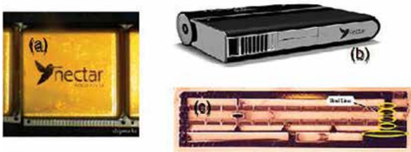
Figure 8. Micro fuel cell and reformer. (a) The packaged reformer; (b) The complete commercial package; (c) A cross section of the interior assembly of the reformer.
